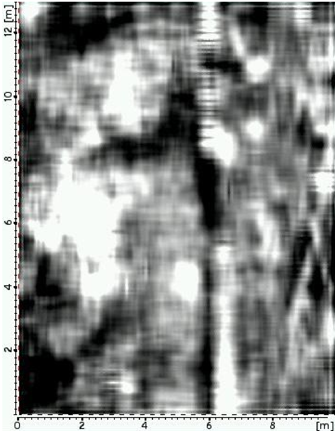
Figure 6.49 – Ground penetrating radar survey of area of OMF 48 [OMF34A]. The stonework is poorly revealed but there is an otherwise unknown East to West buried feature and part of the buried telecommunications line shown in the bottom right. [North is to left of image]
