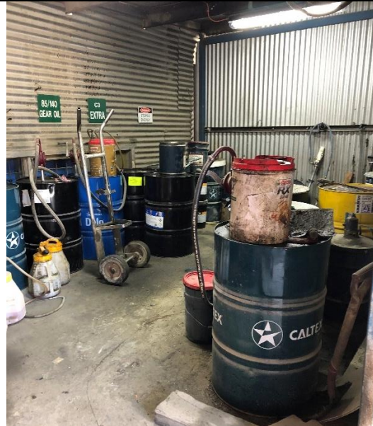
Oil Storage within bunded locked shed
