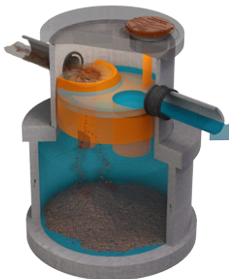
Figure 3 – HumeCeptor® system operation during design flow condition
