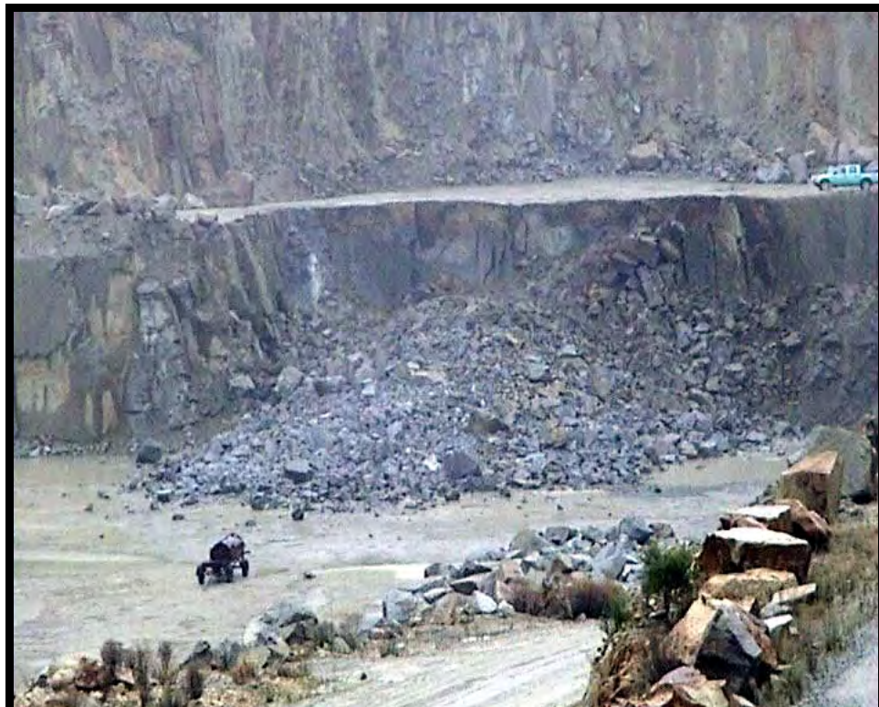
Figure A1.4 – Rock pile left after a blast
