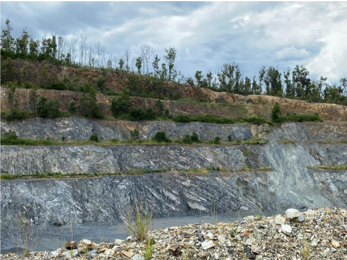
Plate 4 Rehabilitated benches along the eastern side of the AP area.
