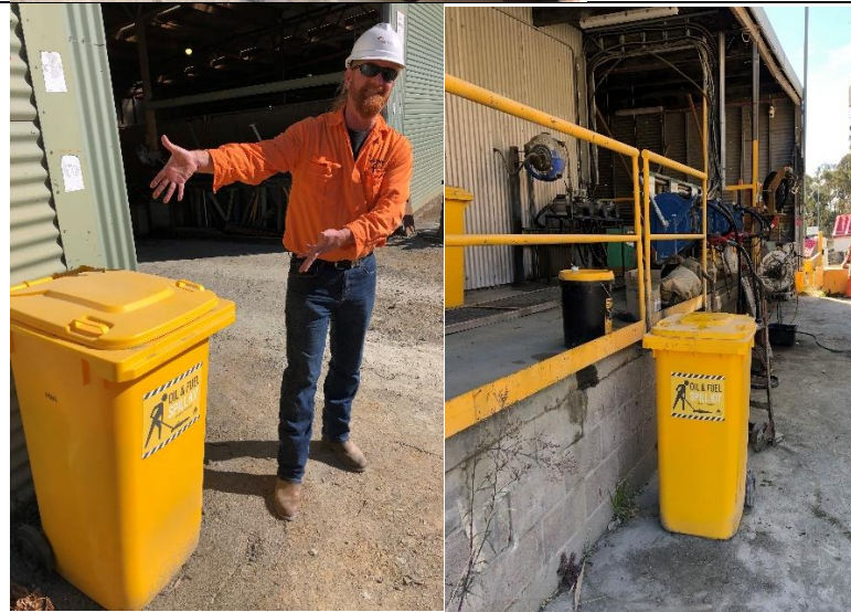
Example of Spill Kits located around site
