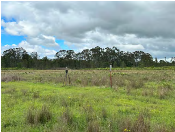
Photograph E.16 Depositional Dust Guage
