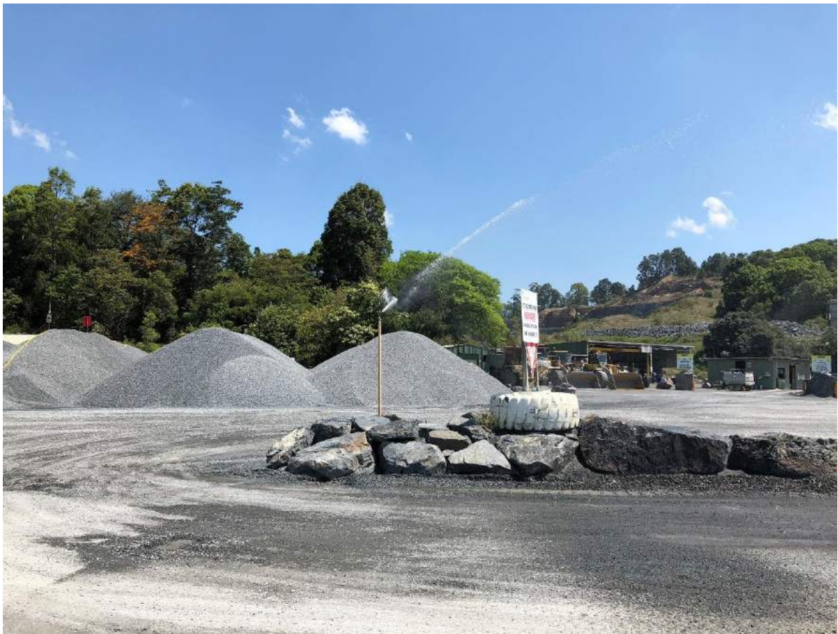
Photograph 14: Dust suppression sprinkler in operation on main driveway
