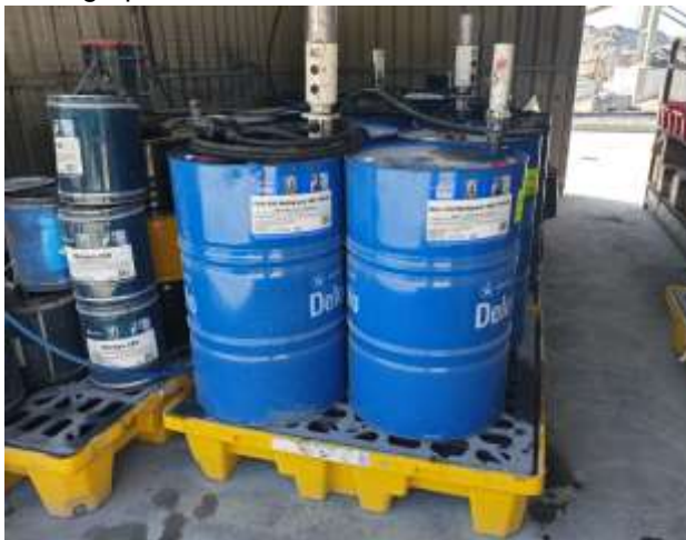
Photograph 7: Bunded fuel and chemical storage
