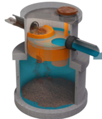
Figure 2 – HumeCeptor® system operation during high flow conditions
