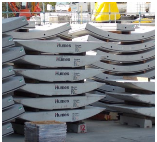
Tunnel invert units
