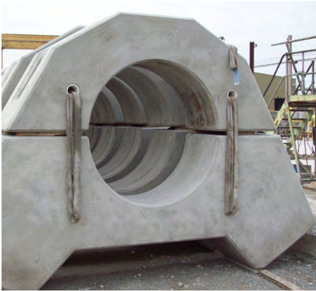
Pipeline anchor blocks
