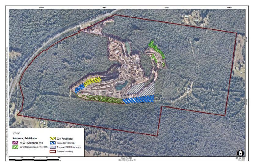
Figure 3: Jandra Quarry Rehabilitation and Disturbance (2018 and 2019)
