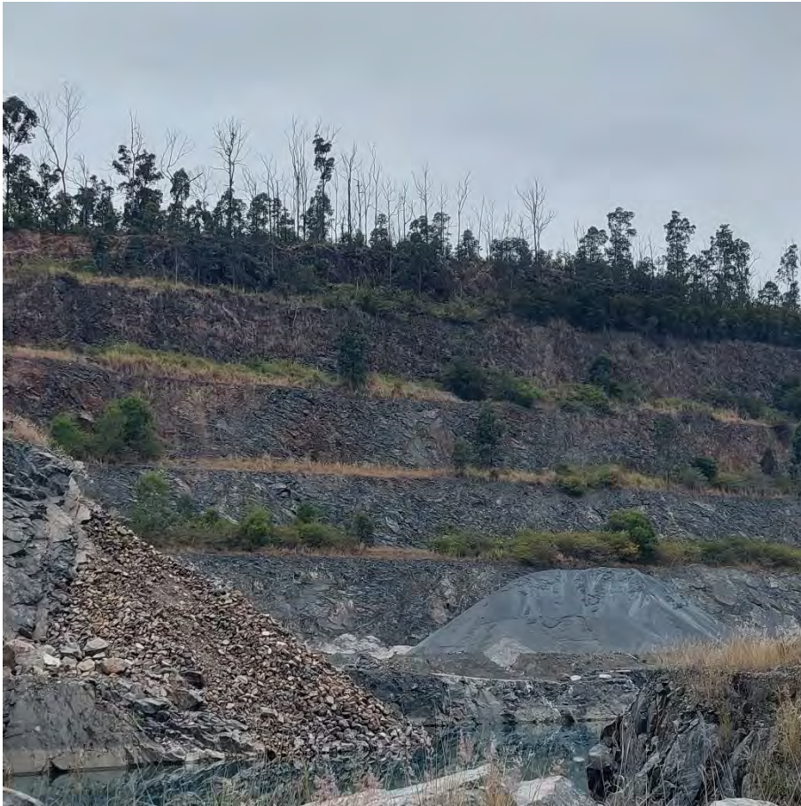
Plate 7 Excavated material perched on edge of settlement dam in the AP area near the ROM 2023 (previously noted in 2022 as falling into dam).
