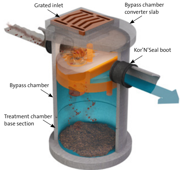
Figure 1 – HumeCeptor® STC2 components
