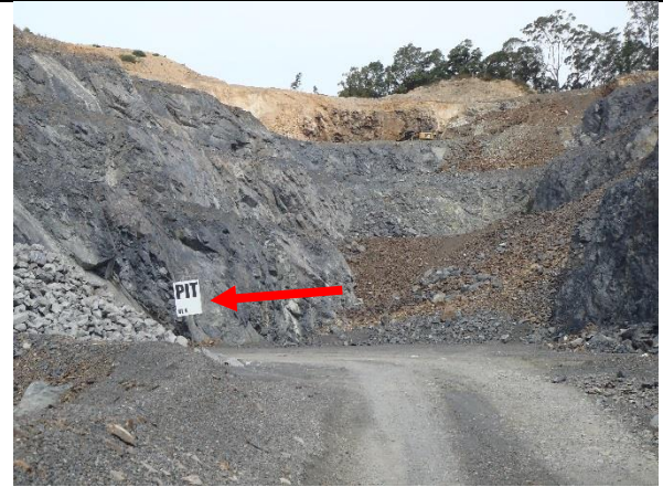
Active quarry pit facing south, showing the area remediated back to RL 4 metres AHD Signage indicates the extraction level of RL 4 metres AHD.
