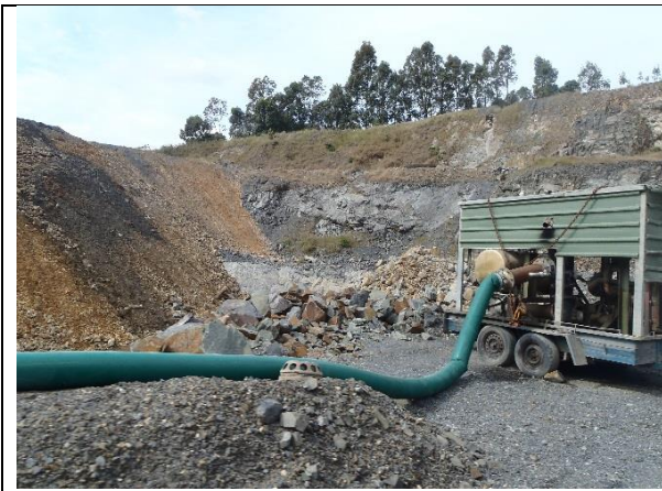
Pump used to transfer water between the Main Dam and in-pit dam.
