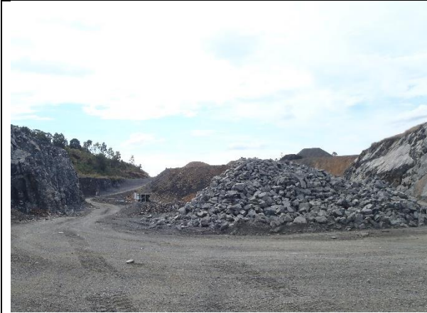
Active quarry pit facing north, showing the area remediated back to RL 4 metres AHD
