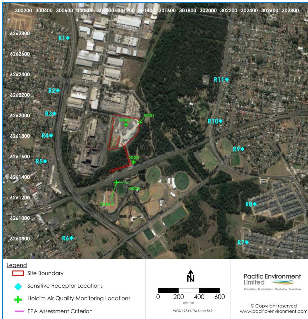
Figure 2-1: Site Location, sensitive receptors and air quality monitoring locations
