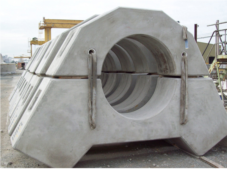
Pipeline anchor blocks
