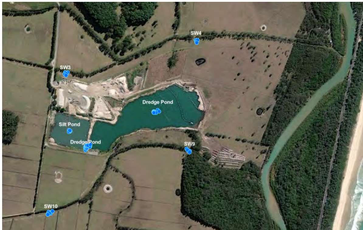
Figure 1-2 Location of Surface Water Monitoring Points
