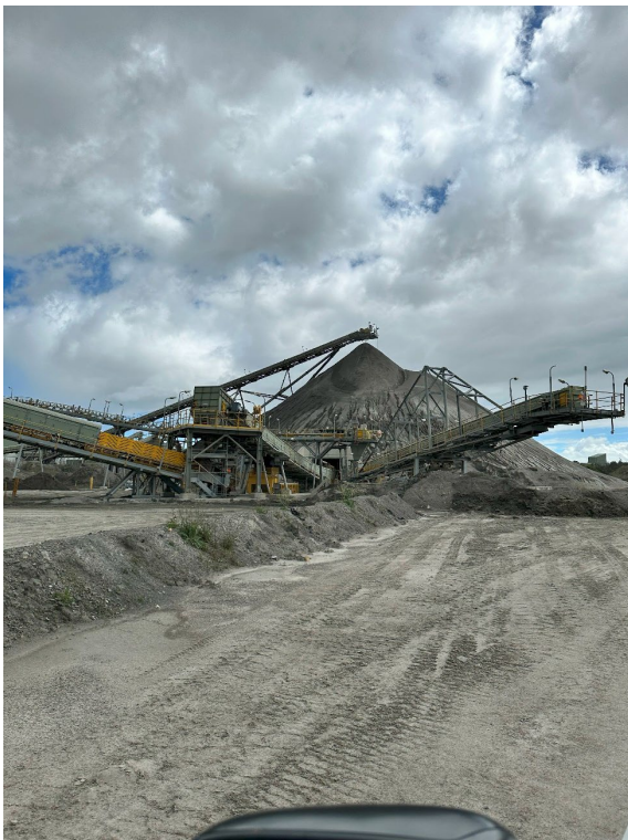
Photograph E.39 Stacker and stockpile
