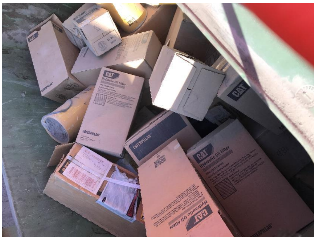
Photograph 21: Used oil filters are being stored in prescribed waste bin inside their cardboard boxes. The cardboard should be segregated and recycled separately.
