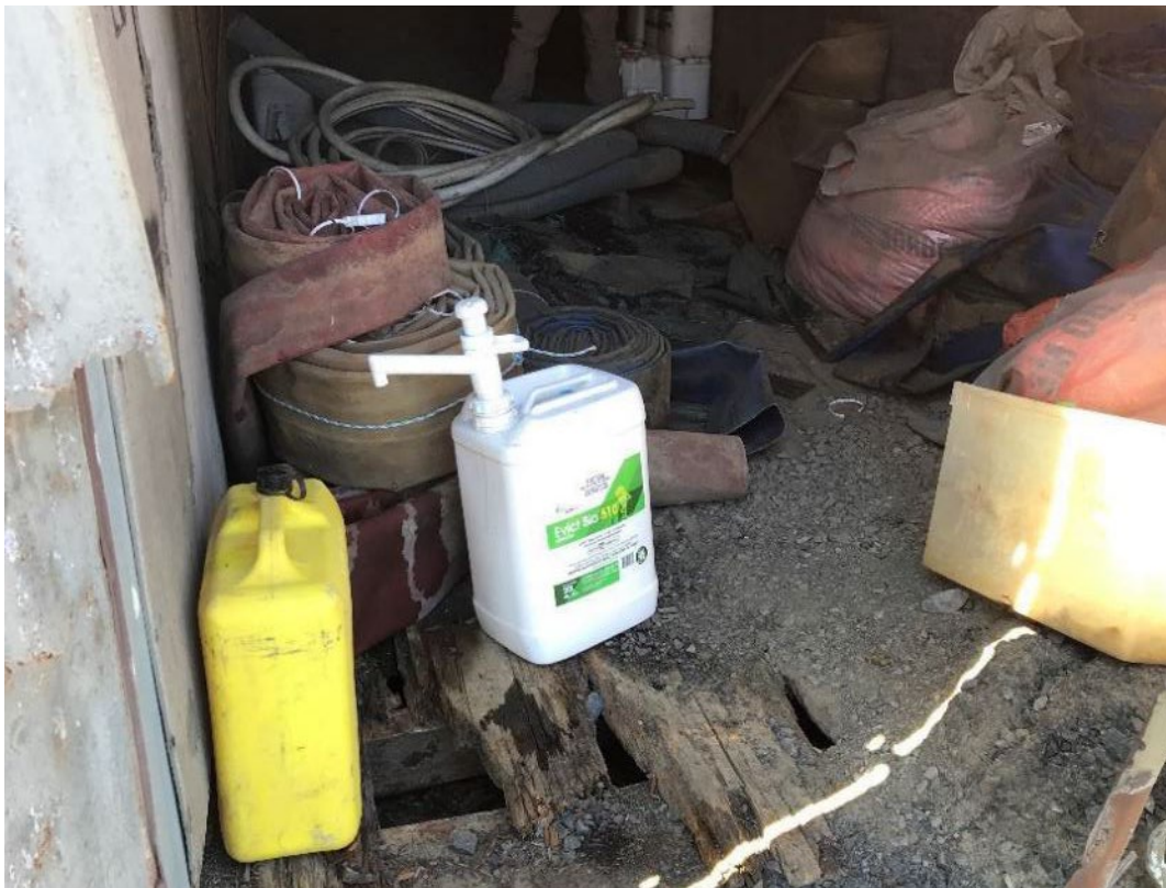
Photograph 17: All chemicals should be contained within bunded areas, or on a bunding pallet.
