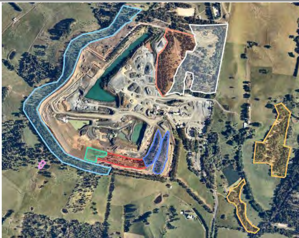
Rehabilitation Areas. KEY: Phase A & B (Teal), 0.8 Hectare (Green), Southern Extraction (Red), South-East Extraction (Blue), Extraction (Orange), Phase C (White), Landslip (Pink) and Net Gain (Yellow).
