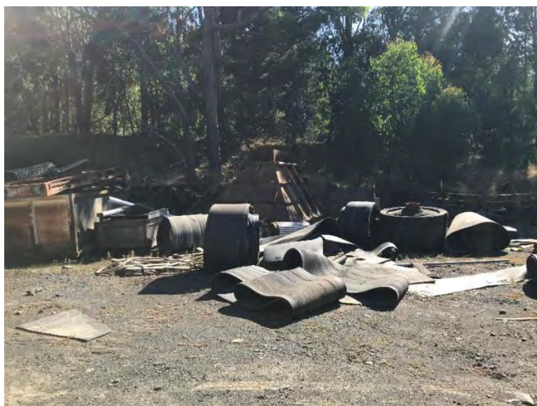
Photograph 21: Waste rubber conveyor belts stored for later re-use/recycle.
