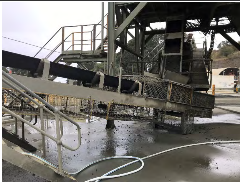
Photograph 65: Cement mixing area, a potential source of elevated pH in the site's surface water system.
