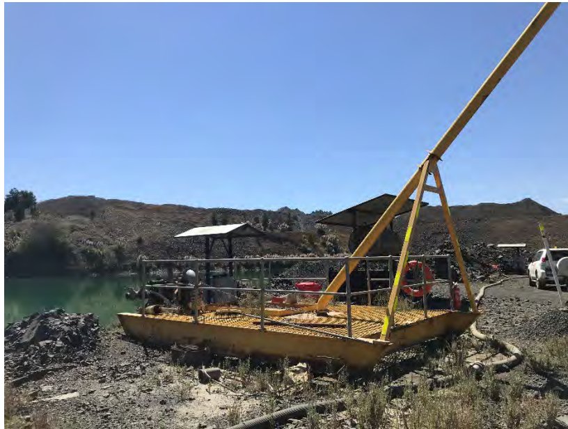
Photograph 51: Pit pumped water offtake and loading standpipe.
