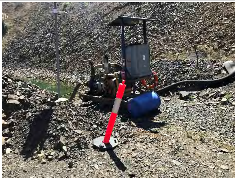
Photograph 55: Main quarry pit – third pump, with spill kit (blue barrel).
