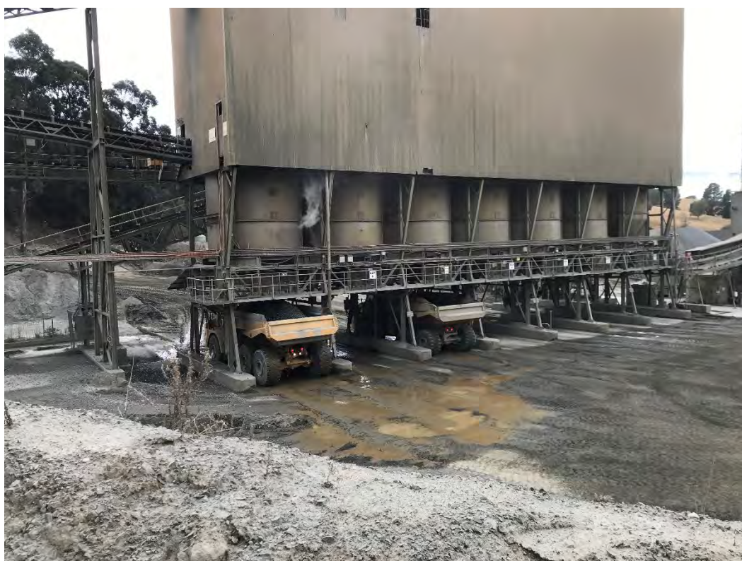
Photograph 16 – Truck load-out area; dust is effectively minimised with water sprays.
