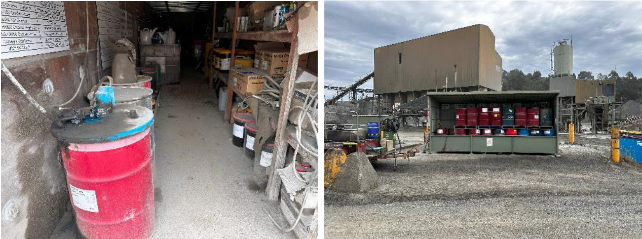
FIGURE 3: GOOD CHEMICAL, FUEL AND OIL STORAGE PRACTICES
