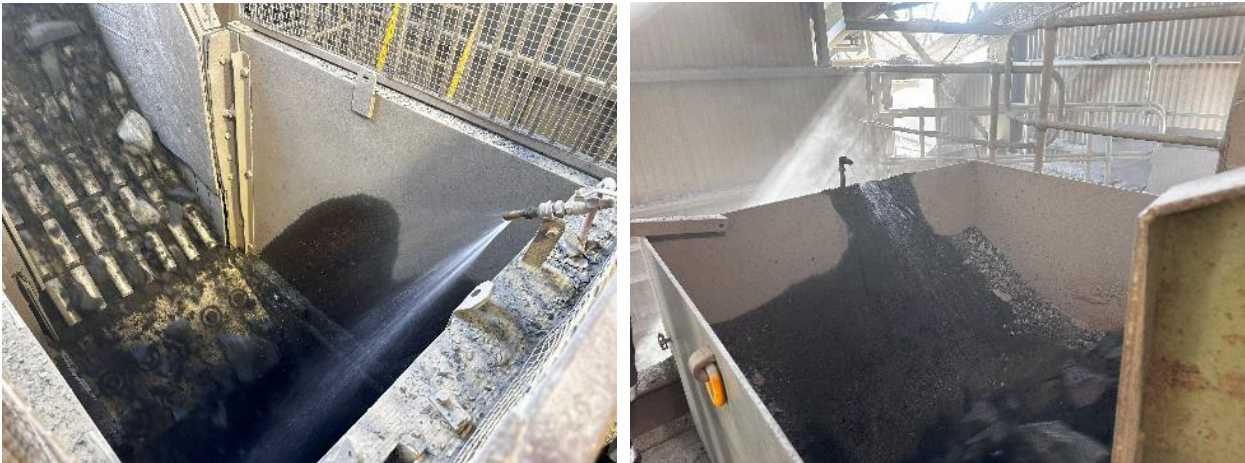
FIGURE 5: WATER SPRAYS OPERATING ON CRUSHING PLANT
