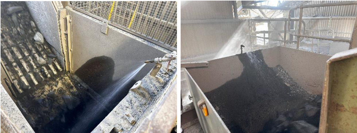
FIGURE 4: WATER SPRAYS OPERATING ON CRUSHING PLANT
