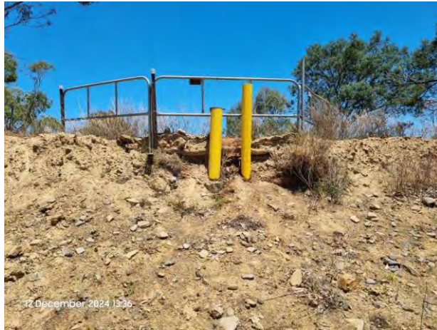
Bore MB01 located at top of steep slope. Monument cover rocks slightly
