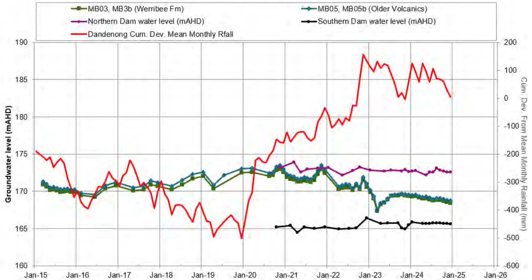
Reduced groundwater levels, bores MB03 and MB06. 2015 to present
