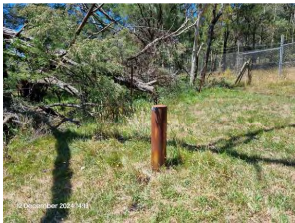
Bore MB06. Steel casing is slightly rusted.
