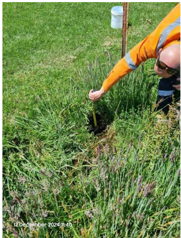
SP08. Measuring water height
