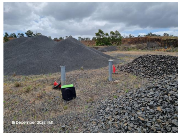
Bores MB02 and MB04 on quarry floor
