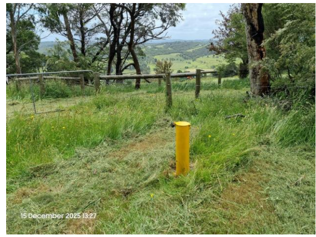
Bore MB06. Steel casing has been repainted. Grass surrounding bore has been slashed to aid access.
