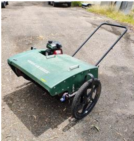
Picture 1. Grass Grabber, a manually propelled seed harvester
