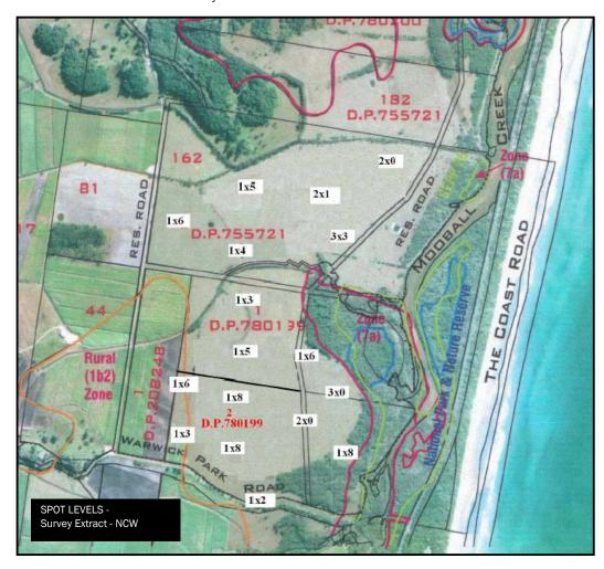
The extraction areas proper are generally limited in elevation to between 1.3m AHD and 2.0m AHD.
