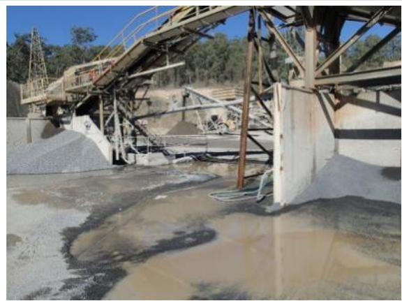
Crushing and screening plant, with wash down occurring to minimise dust issues.
