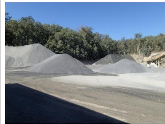
Product stockpiles, with a sprinkler system operating on the stockpile in the back, right.
