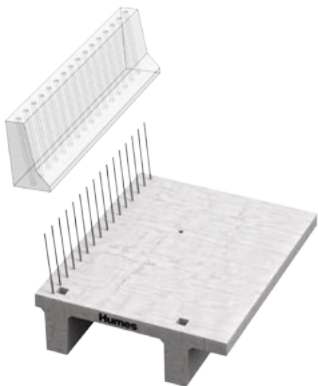
Figure 13 – Concrete barrier fixing
