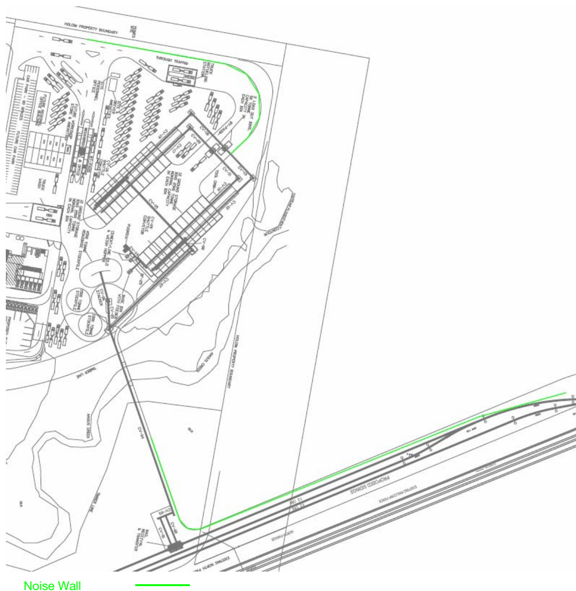
Figure 1 Noise Wall Locations
